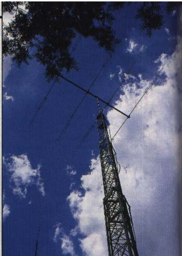
WB6ACU's connection with the ham radio world — a KLM KT-34 beam at 60 feet.
